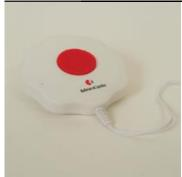
Device placed under users pillow and vibrates to wake upon linked alarm / alert (see other Bellman items in this catalogue section such as smoke alarms and push button transmitter).
